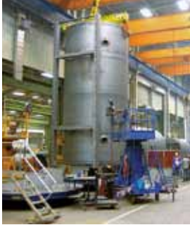
Welding the pressure vessel in the optimum welding position
