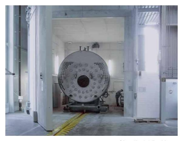
Boiler assemblies and entire Vitomax boilers are inspected for fault-free weld seams and material weakness inside the X-ray chamber.
