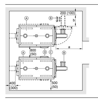
To enable convenient installation and maintenance, observe the stated clearance dimensions; where space is tight, only the minimum clearances (dimensions in brackets) need to be maintained. In the delivered condition, the boiler door opens to the right. The hinge pins can be repositioned so the door swings open to the left.
