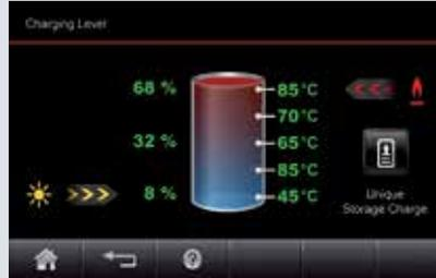
**Temperature stratification in the cylinder**
